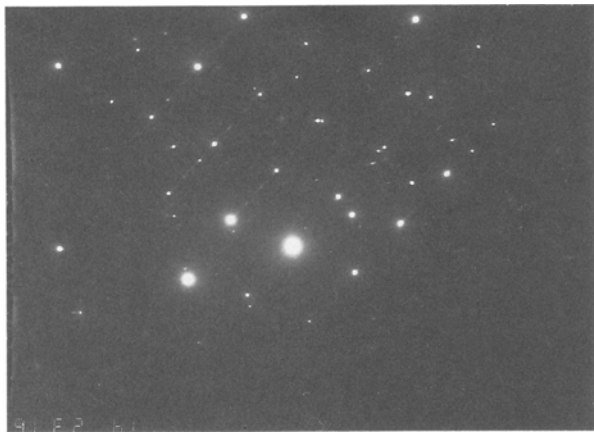
Figure 6 Electron diffraction pattern for a film deposited at 630 °C and 24 Pa.
