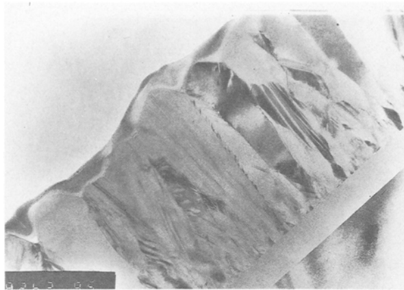
Figure 15 Cross-sectional TEM micrographs for films deposited at 590 °C and 0.33 Pa.
