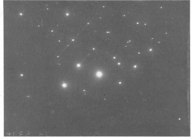
Figure 12 Electron diffraction pattern for a film deposited at 630 °C and 0.33 Pa.
